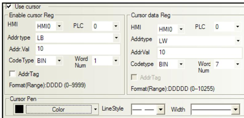
As following picture: Set Enable Scroll Address LB0 to ON, then Scroll Data Address LW10, LW11, LW12, LW13, LW14, LW15 correspond to second, minute, hour, date, month, and year of the sampled data respectively. LW16 corresponds to data value of channel 0; LW17 corresponds to data value of channel 1, and so on.
