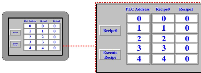
Press [recipe 0] button and switch to [recipe 1], and modify the value of PLC address 4X1~4X5 to 5~9, then press [Execute Recipe] button, the value of RW5~RW9 will display 5~9.
