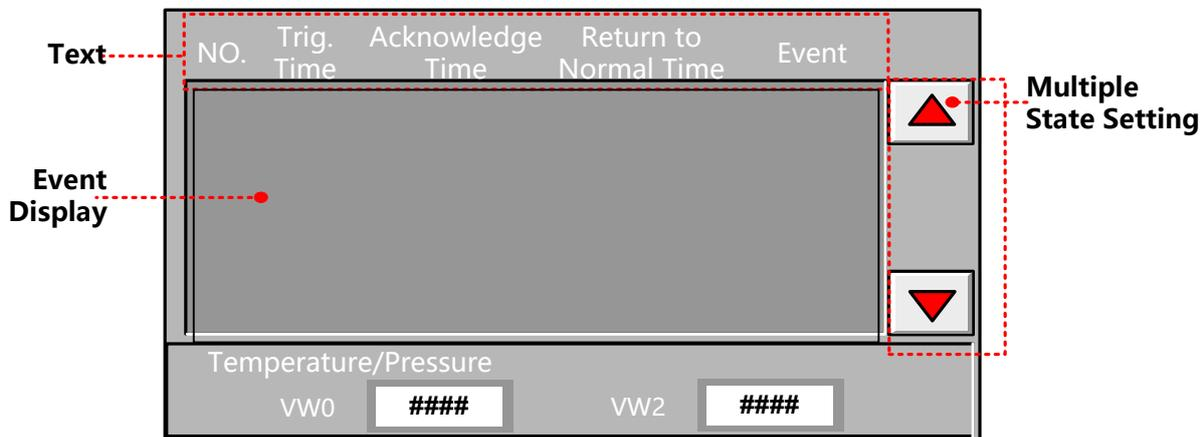
① Create new project [Event], and then add two windows Frame10 and Frame11 which are used for temperature alarm and pressure alarm. Set the attributes as follows:
