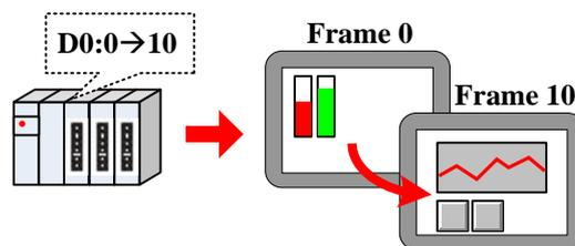
For example, Suppose the current window number is 0, specified register address is D100, when the D100 is 10, the HMI switches to the window 10, and return the new window number 10 to D101.
