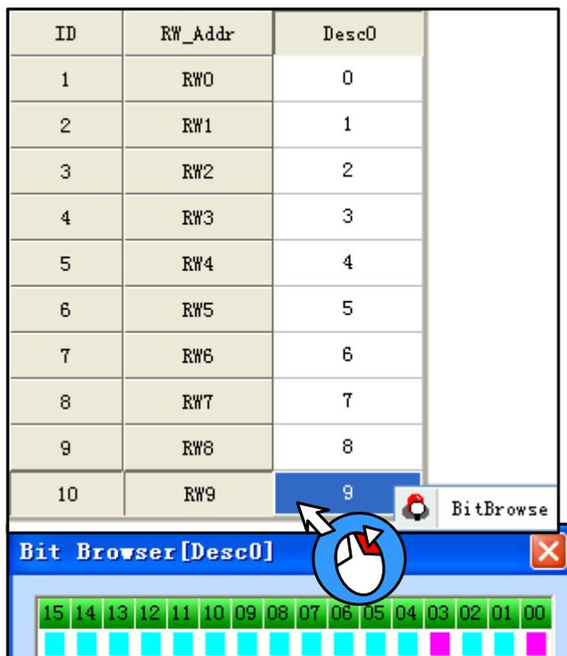
[Examples] For example RW9 value is 9, bit browser form RW9: 03,00 bit address can be seen in red: ON, decimal 9 to binary form as 0000 0000 0000 1001.
