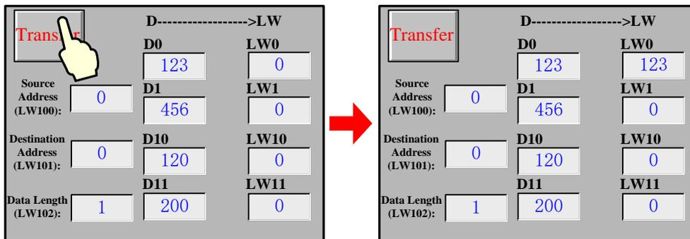
When the offset of Source Address is 10, offset of Destination Address is 10 and the Data Length is 2:
