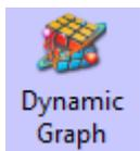
Dynamic Graph can change the position and size of rectangle, ellipse or line according to value in the specified HMI/ PLC register.
