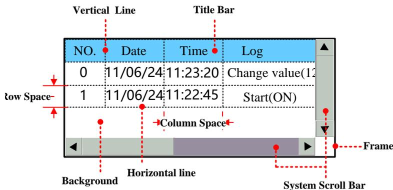
\* When the operation log cannot be wholly displayed in vertical or horizontal direction, system will provide scroll bar automatically. The width of system scroll bar can be set in HMI Extend Attributes of HMI Attributes; the width is optional from 20 to 120(pixel).
