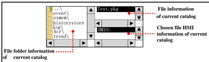
File list component is a special component; it is usually used together with the Import/Export function of Function Key. System also provides [Frame5: File List Window] as file list when user import/export project file or recipe file in the SETUP screen. And the File Browser Window can be changed in the HMI Attributes.
