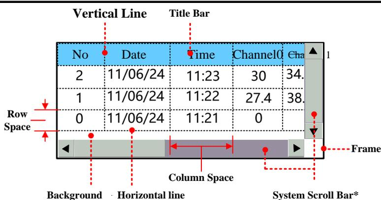
※If the information in Historical Data Display component cannot be displayed entirely, the scroll bar will be built automatically to make user to view the whole information. And the width of system scroll bar can be set in HMI Attributes >> HMI Extended Attributes, ranges from 20~120 pixel.
