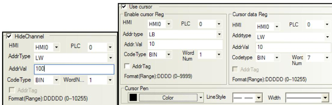
Set LW. B100.0 to ON, Channel 0 will be hidden; Set LW. B100.1 to ON, channel 1 will be hidden and so on.
