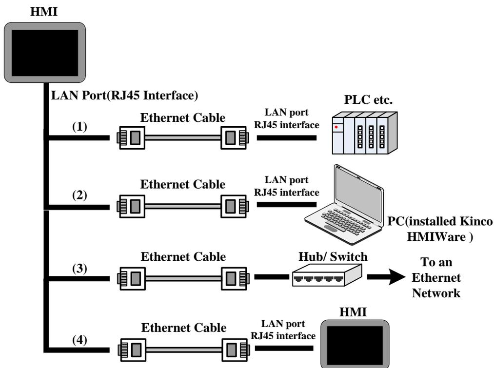
(1) Connect with PLC and such controllers to communicate
