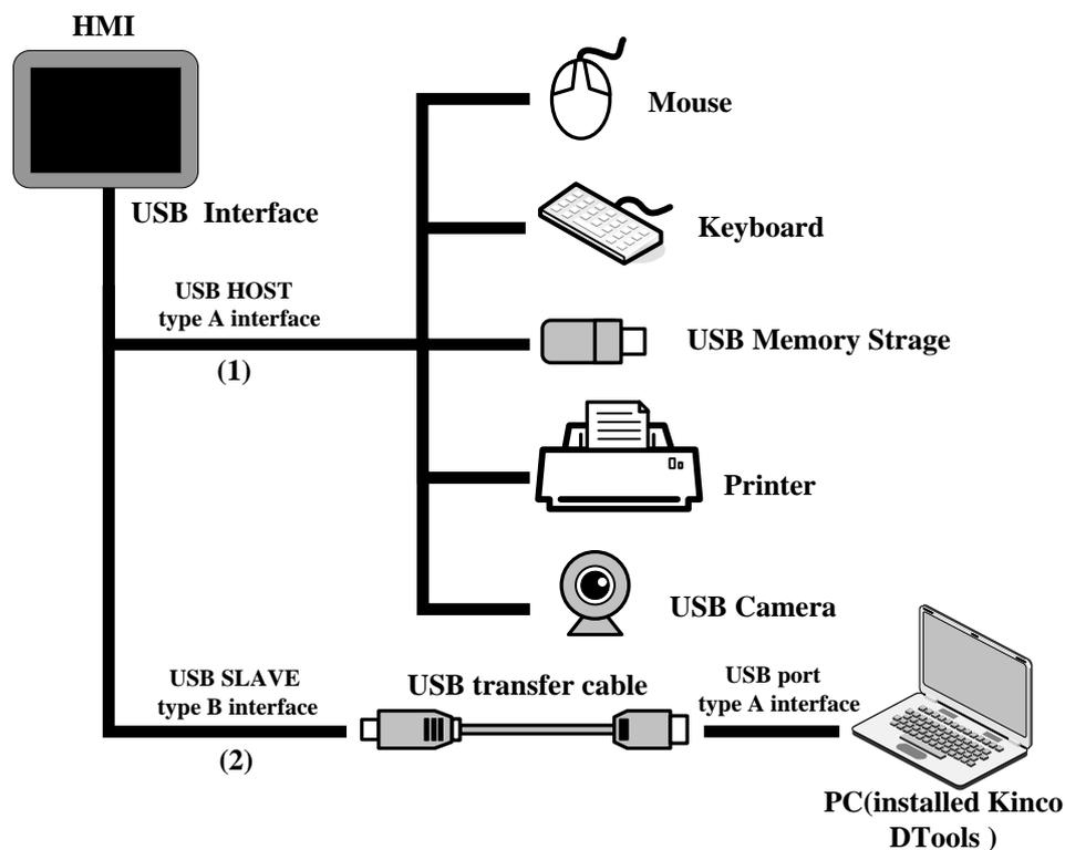
(1) Connect with USB mouse, USB keyboard and such equipment via USB HOST
