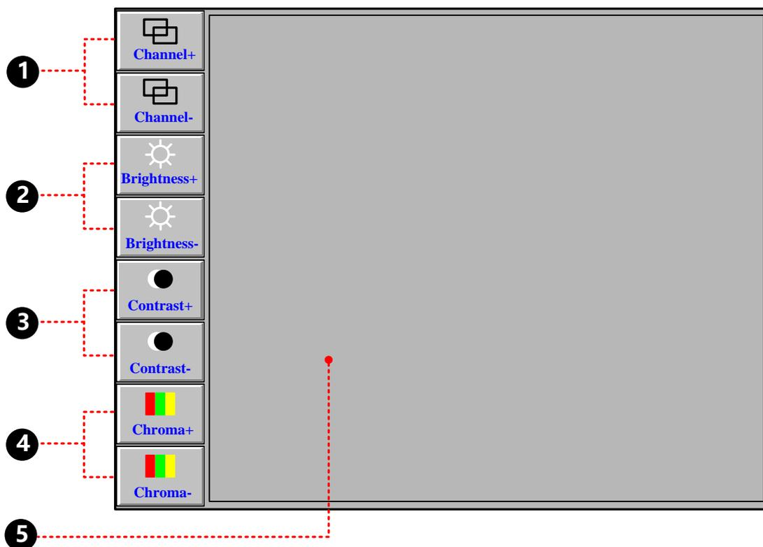
① Multiple State Setting component, it is used to switch the channels (There are only 2 CVBS port on MT5620T), its
