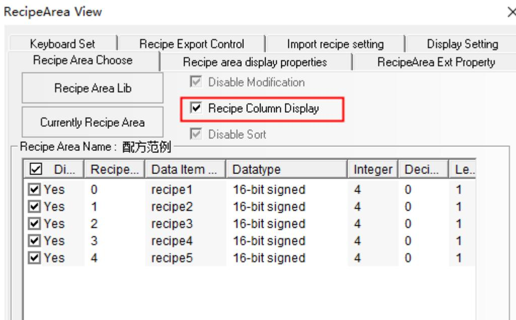
2.The left column shows the list of recipe parameters, and the right column shows the corresponding recipe content.
