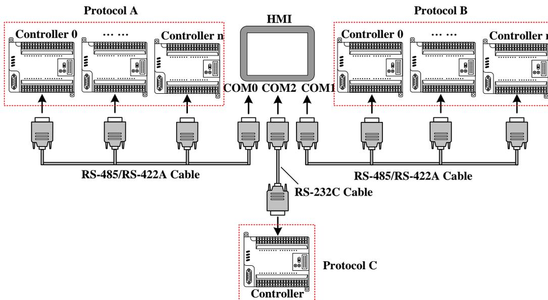
[Example] Below a GH070E with three MODBUS device (hereinafter referred to as PLC 0, PLC 1, PLC 2), a MITSUBISHI FX2N (hereinafter referred to as PLC 3), an OMRON CP1H (hereinafter referred to as PLC 4) communication is cases, Requirements were monitored on the HMI PLC 0, PLC 1, PLC 2 of 4X 100, PLC 3 of D100 data and PLC 4 of Q 0.0 outputs.
