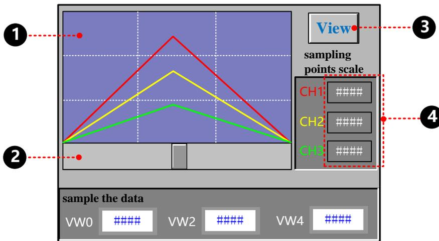
① Build a new Trend Curve component, the component attribute is as followings:
