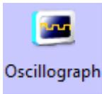
The function of Oscilloscope component is similar to the Trend Curve. They read continuous registers from specified HMI local registers or PLC/Controller registers periodically, and plots them in single axis curve.
