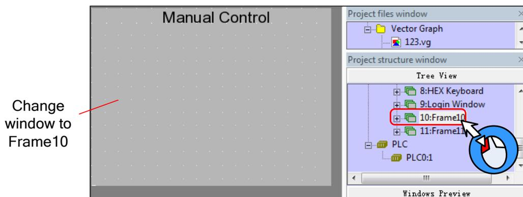
Add 8 “Bit State Switch” components from **Graph element window** — **PLC Parts** for controlling the start and stop of electric valve, metering pump, circulating pump and air blower.
